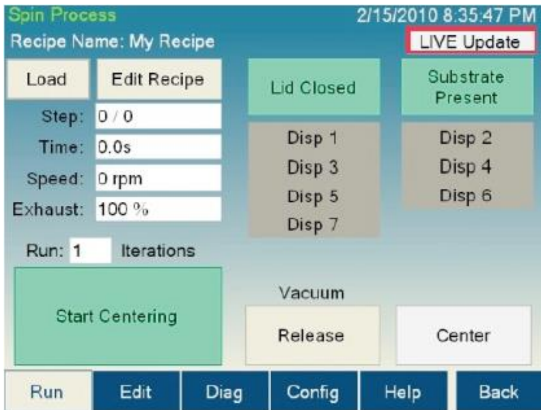
recipe while its running. The LIVE Update feature is not available on all models. Figure 7.1 Spin Process Page with LIVE Update button highlighted
