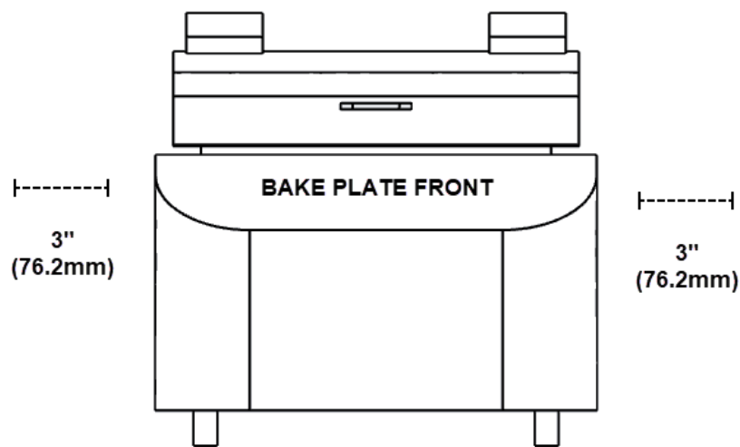
Figure 2: Apogee® 300 Bake Plate Side Clearance Requirements
